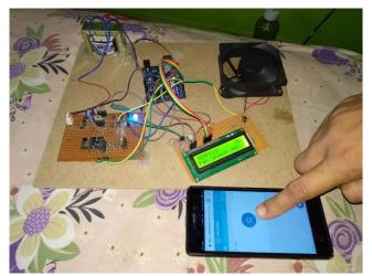
Fig. 9 Fan is switched using mobile phone
