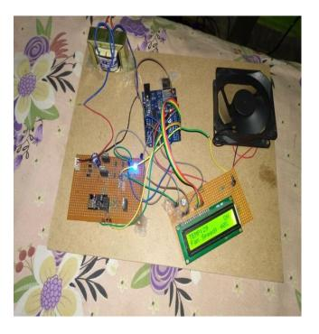
Fig.11 Temperature 29°C and Fan running at 40% of its full speed.
