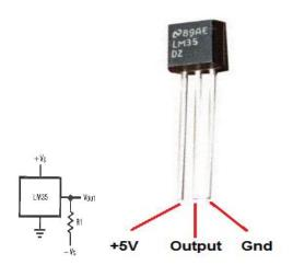
Fig.2: LM35 Temperature Sensor B. ESP8266 WI-FI MODULE:
