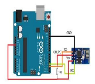
**Fig.5** connecting Arduino and Esp8266. By connecting Arduino and ESP8266 as shown in the above fig.(5) program can be dumped into the Wi-Fi module.
