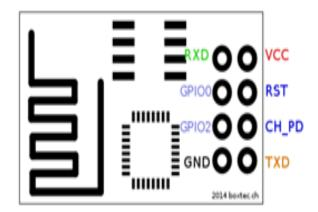
**Fig.4:** Pin diagram of ESP8266 01 Wi-Fi module Connect arduino with ESP8266 as follows Arduino —— ESP8266
