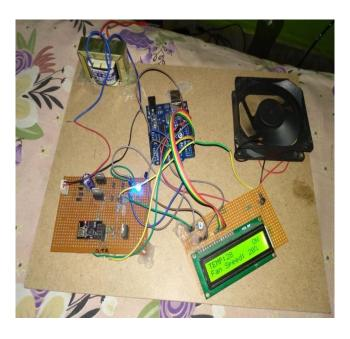
Fig. 10 Temperature 28° C and Fan running at 20% of its full speed.
