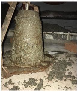
Figure 4: Slump test
