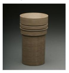
Fig.2 Fiberglass reinforced composite insulating sleeve. In this case the fiber was chosen for its insulating properties and strength to transfer loads between metal components.
