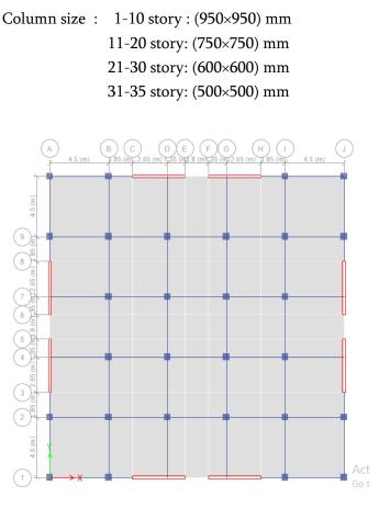
Figure 2: Plan of a structure
