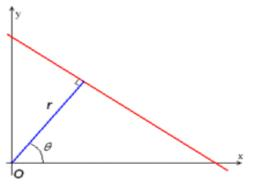
Figure 6: Hough Transform
