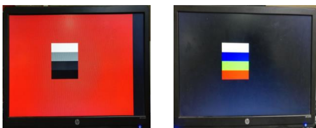
Figure 4: Fixed pattern generate from FPGA
