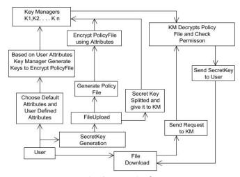
FIGURE 1: System Architecture
