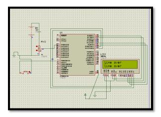
**Figure6:** As per the time setted till there the charging is done and then it stops charging and displays the message "time over".
