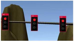
Figure 1: Traffic Light Detection
