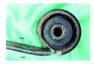
**Fig. 2** The broken halves of the spring have been placed together in a manner exaggerating the opening of the eye before rupture<sup>(3)</sup>
