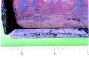
Fig. 3 The spring half of the fracture has deep secondary cracking along the midplane<sup>(3)</sup>
