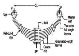
Figure-1: Main parts of Leaf Spring<sup>(3)</sup>
