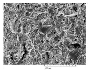
Fig. 4 This fracture area is approximately halfway between the inside spring surface and the midplane fracture<sup>(3)</sup>
