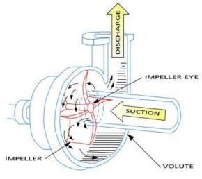
Figure 1 – Centrifugal Pump
