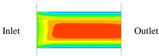
Figure 3.1.4 VELOCITY PROFILE SECTION VIEW
