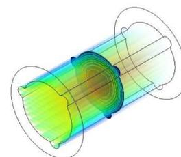
Figure 3.1.2 VELOCITY CONTOUR AT CENTRE
