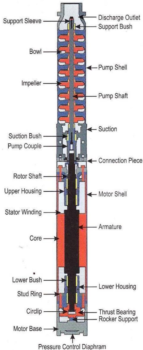
For motors above 1.0 hp, it experienced bearing bush failure after just few months of operation. Where as its earlier products i.e. 150 mm and 200 mm submersible motors operated smoothly for more than
