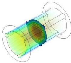
Figure 3.2.2 VELOCITY CONTOUR AT CENTRE
