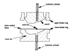
Figure 1- Tailor Welded Blank
