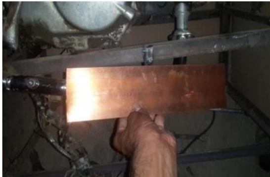
Figure 5 Copper heat source fabricate for the present study
