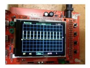
Figuer 3. Harwared Based Waveform By Cro
