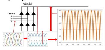
**Figure 1** Rectifier circuit and waveforms
