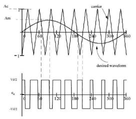
Figure 2. Pulse width modulation technique
