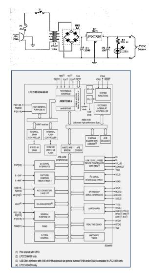
Figure 1: 5V dc Circuit Diagram & LPC2148 block diagram
