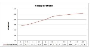
Figure 3. temp v/s time when peltier is heating
