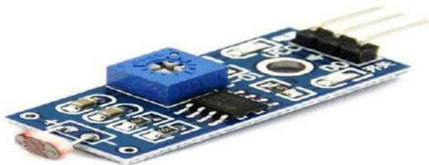
Figure 9. Ldr (Light Dependent Resistor Module)
