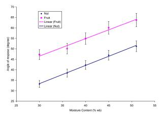
Figure 6: Effect of moisture content on the angle of repose gmelina fruit and nut
