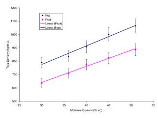
Figure 4: Effect of moisture content on the true density of gmelina fruit and nut.
