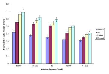
Figure 7: Effect of moisture content on the static friction of gmelina fruit
