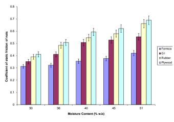
Figure 6: Effect of moisture content on the static friction of gmelina nut
