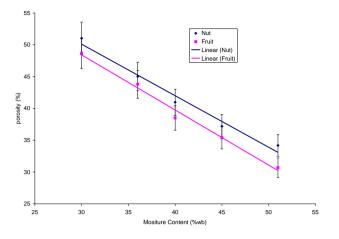
Figure 5: Effect of moisture content on the porosity of gmelina fruit and nut.
