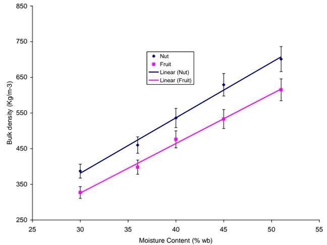
Figure 3: Effect of moisture content on density of gmelina fruit and nut.
