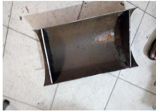
Figure 2. Fabricated Reinforcement plates
