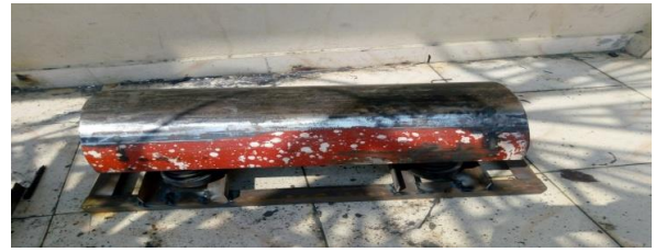
Figure 6 . Assembly Of Speed Breaker
