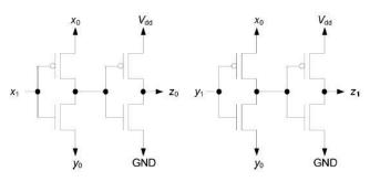
Figure.4: Two-pair two-rail checker
