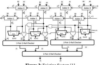
3.1 Design of A Self-Checking 2-Bit Carry-Select Adder
