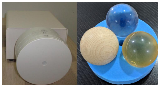
Figure 1. Anzai AZ-7332 respiratory monitoring system a) motion phantom and b) Different Inserts
