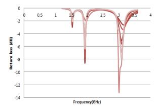
Figure 2. Parametric analysis of varying Coaxial feed positions-Reflection Coefficient of the Proposed Antenna.
