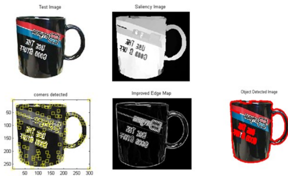
Figure 2. Test image is uploaded, then it finds an salient region, corner detection and edge detection
