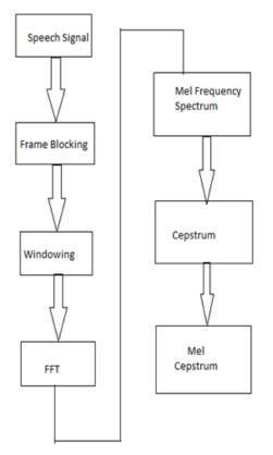
Fig -2: MFCC Block Diagram
