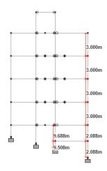
Fig 4.12 . Elevation of residential building on 15 deg. Slope
