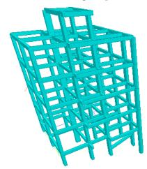
Fig 4.2.2 . Structural model of building on 15 deg. slope
