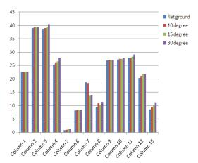
Above graph shows the maximum shear force in Zdirection is increases with increasing the slope of ground.
