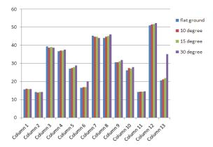
Above graph shows the maximum bending moment in Z-direction is increases with increasing the slope of ground
