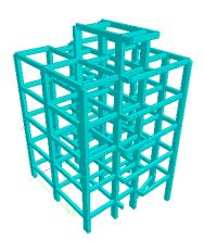
Fig 4.2.2 . Structural model of building on 10 deg. slope
