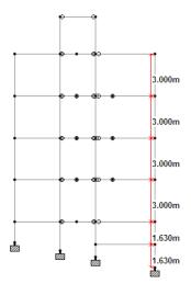
Fig 4.2.1 . Elevation of residential building on 10 deg. Slope
