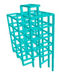
Fig 4.2.2 . Structural model of building on 30 deg. slope
