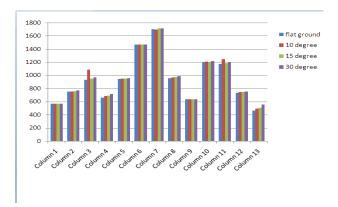
Above graph shows the maximum axial forces is increases with increasing the slope of ground
