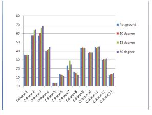
Above graph shows the maximum bending moment in Y-direction is increases with increasing the slope of ground
