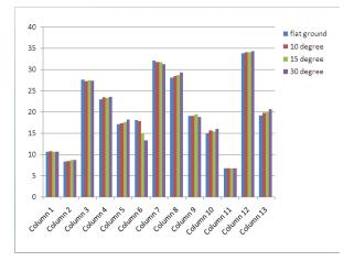
Above graph shows the maximum shear force in Ydirection is increases with increasing the slope of ground.
