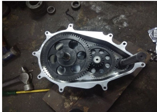
Figure 1. Open gearbox casing
