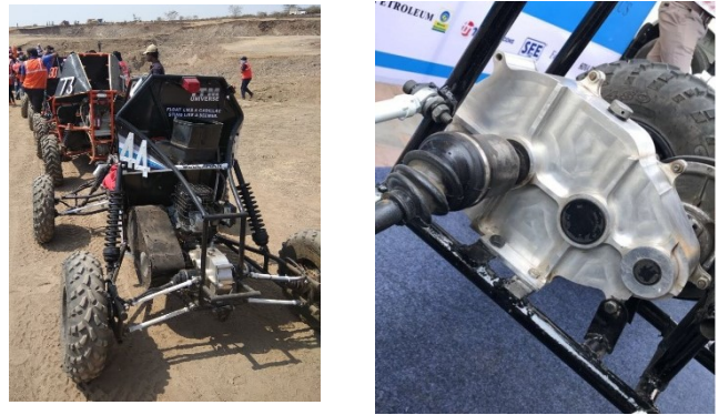
Figure 26. Actual mounting of gearbox on vehicle
