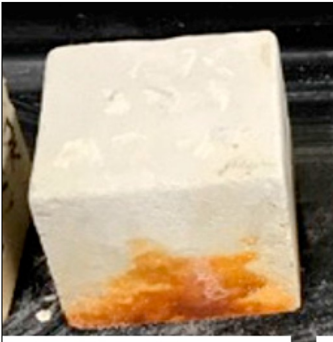
Figure 3: A sample specimen Sulfate Attack
