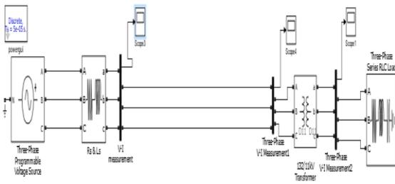
**Figure 5.** Simulation of 132kV transmission line without STATCOM
