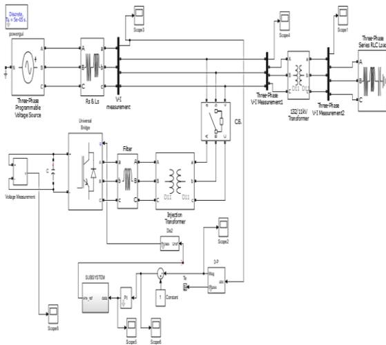
**Figure 6.** Simulation of 132kV transmission line with STATCOM
