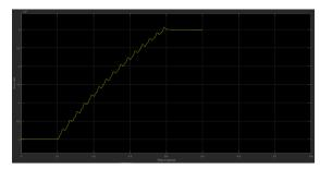
Figure 10. Waveform of voltage across capacitor during compensation of voltage swell by using STATCOM
