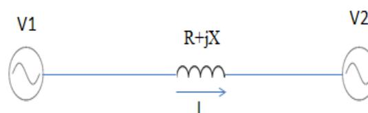
Figure 1. Block diagram of active or reactive power transfer.
