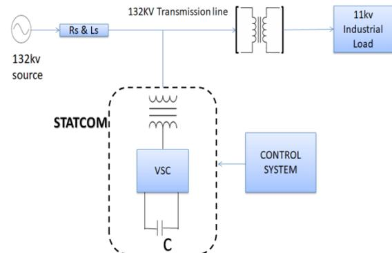
**Figure 2.** Block diagram of transmission line with STATCOM
