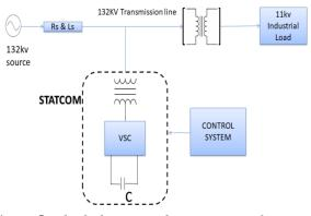
Figure 2. Block diagram of transmission line with STATCOM
