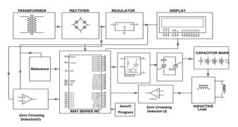
Figure 1. Block diagram of reactive power compensation technique
