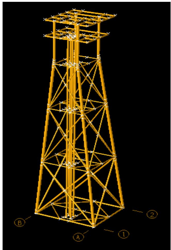
**Figure 1.** 3D Model in SACS
