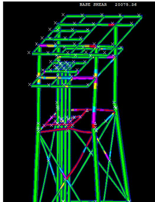
**Figure 2.** Collapse Platform.
