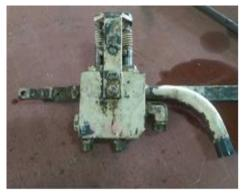
Figure 7: Directional control valve
