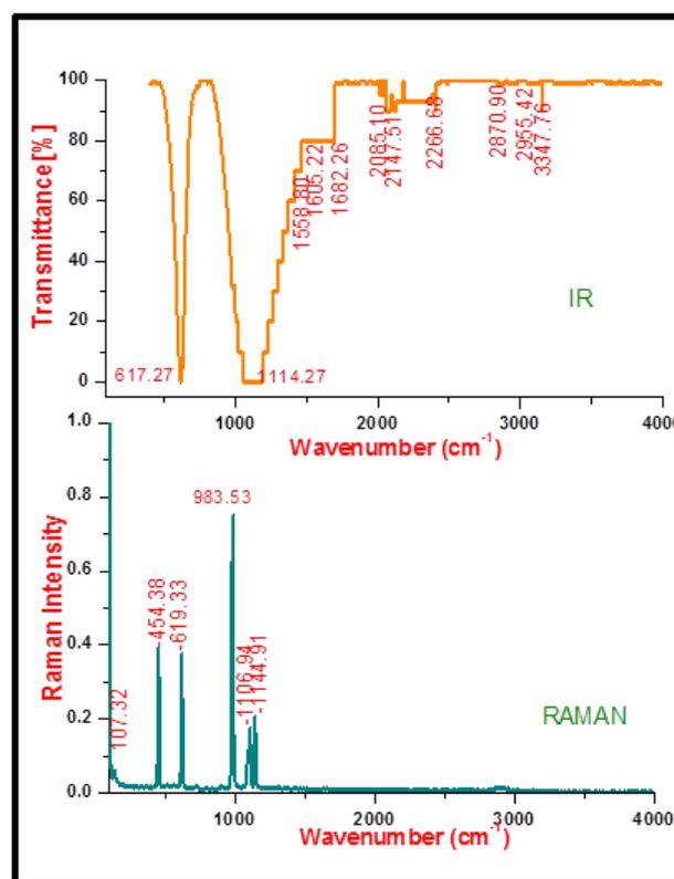
**Figure 4.** IR and RAMAN spectra of LAKS crystal
