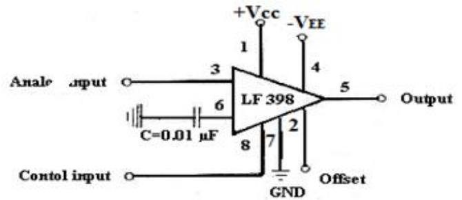
Figure 3. Connection diagram of LF 398 IC
