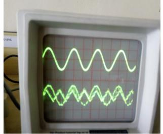
(c) Message Signal and PAM-TDM output **Figure 8.** Generation of PAM-TDM
