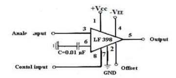
Figure 3. Connection diagram of LF 398 IC
