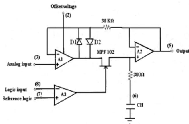
Figure 2. Functional diagram of LF 398 IC
