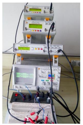
(b) FSK Implementation and Its Output Waveform Fig. 10. FSK Waveform Generation
