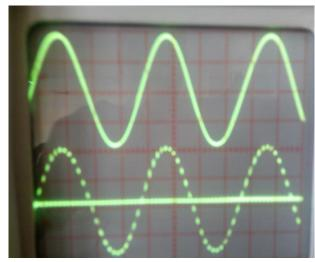
(c) Message Signal and PAM Output Waveform **Figure 5.** Generation of PAM Output Waveform
