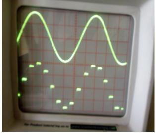
(c) Message signal and Flat top sampling output waveforms Fig.7. Generation of flat top sampling waveform
