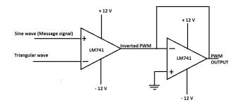
(a) Pulse Width Modulation (PWM) Circuit
