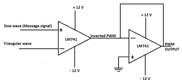
(a) Pulse Width Modulation (PWM) Circuit
