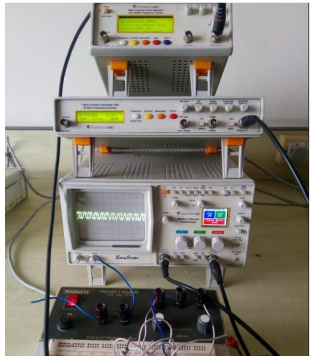
(b) PSK Implementation and Its Output Waveform
