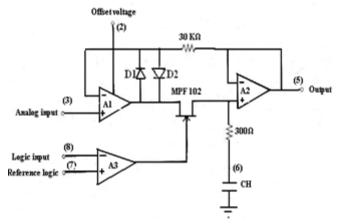
Figure 2. Functional diagram of LF 398 IC
