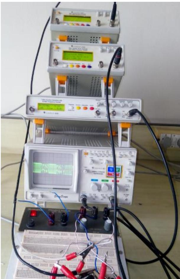
(b) FSK Implementation and Its Output Waveform
