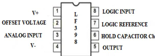
Figure 1. Sample and Hold LF 398 IC
