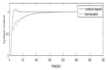
Figure 4. Step Response for P<sub>2</sub>(S) For the Considered Anti-Windup Schemes
