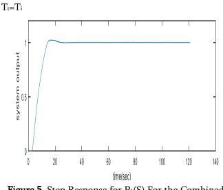
Figure 5. Step Response for P<sub>1</sub>(S) For the Combined Anti-Windup Schemes
