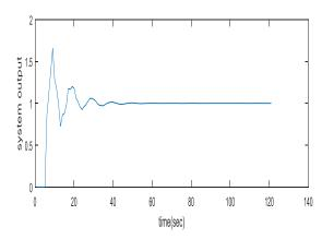
Figure 8. Step Response for P2 (S) For Without Anti-Windup Schemes
