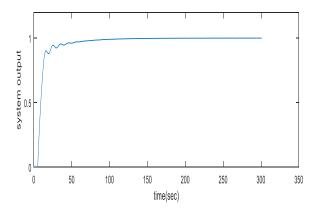
Figure 6. Step Response for P<sub>2</sub>(S) For the Combined Anti-Windup Schemes
