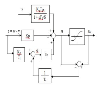
Figure 2. Anti-Windup scheme of Back-Calculation
