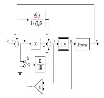
Figure 1. Anti-Windup Scheme of Conditional Integration.
