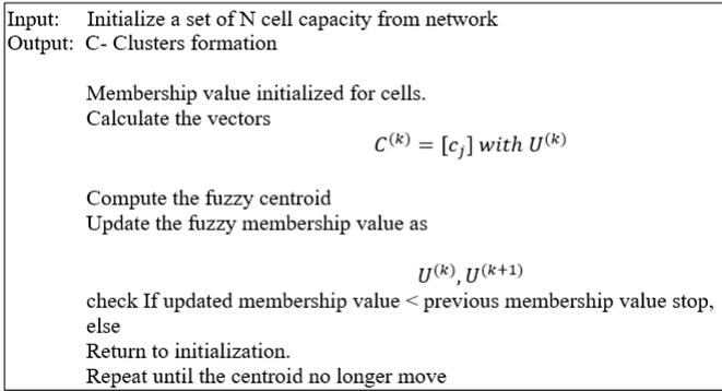
**Figure 2.** Algorithm for proposed FCM based DSA
