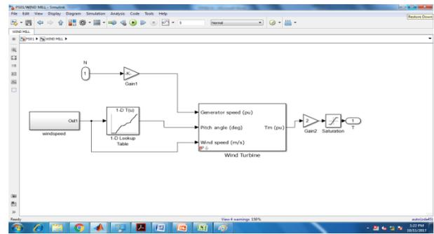
This is the wind turbine model in which the generator speed, pitch angle, wind speed is calculated.
