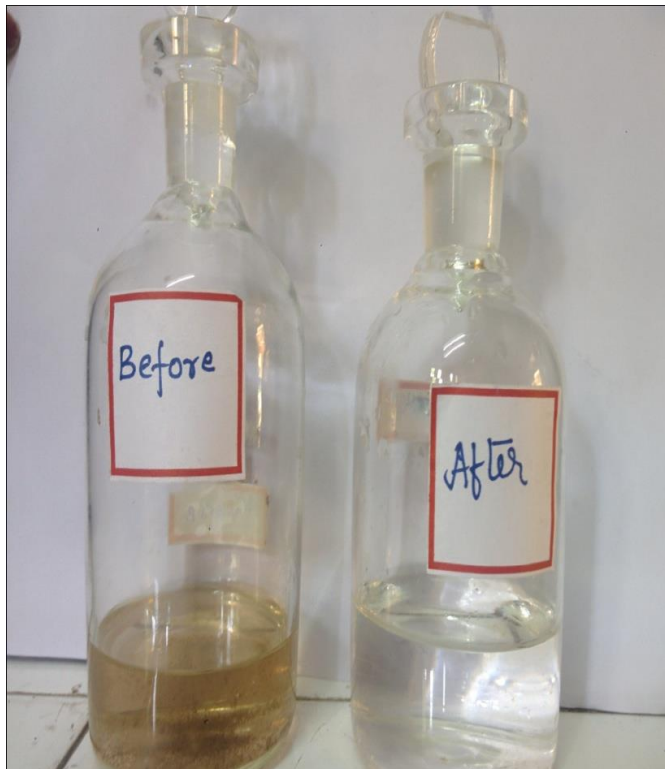
Fig 6 Colour comparison of the effluent before and after treatment
