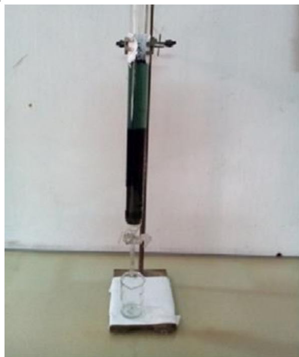
Fig 2 Experimental column packed with MWCNTs
