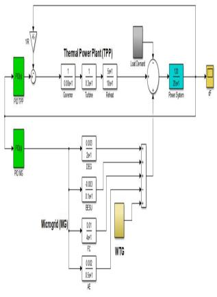
Figure 1. MATLAB Simulation model of a hybrid power system
