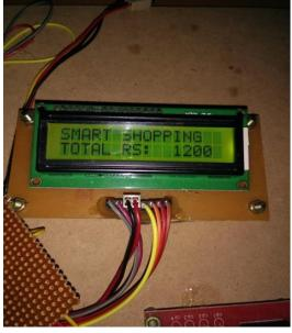
Figure 11. Displaying cost of the product on LCD
