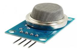
Figure 3. MQ6 gas sensor
