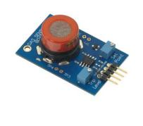
Figure 2. MQ7 gas sensor
