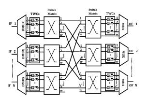
Figure 2: The OBS core node model flowchart
