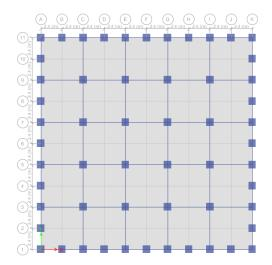
Figure 2: Plan of Framed Tube Structure
