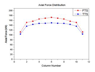
Figure 7: Axial Force variation of periphery columns of Buildings
