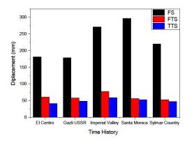
Figure 1: Max. Lateral Displacement of Buildings
