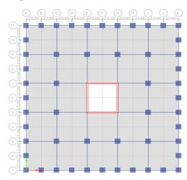
Figure 3: Plan of Tube-in-tube Structure
