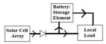
Figure 1: Basic solar (photovoltaic) electric power generation system
