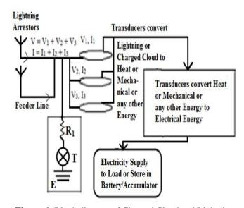
**Figure 6:** Block diagram of Charged Cloud and Lightning electric power generation system with parallel plate transducers.
