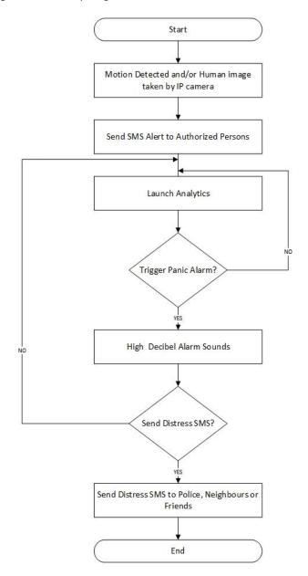
**Figure 3 :** Flowchart of Implemented Analytics Based Anti-Intruder Monitoring and Alarm System.
