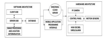
**Figure 1 :** Overall System Architecture
