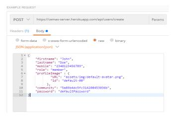
Figure 5: A test request sent for Create User Service
