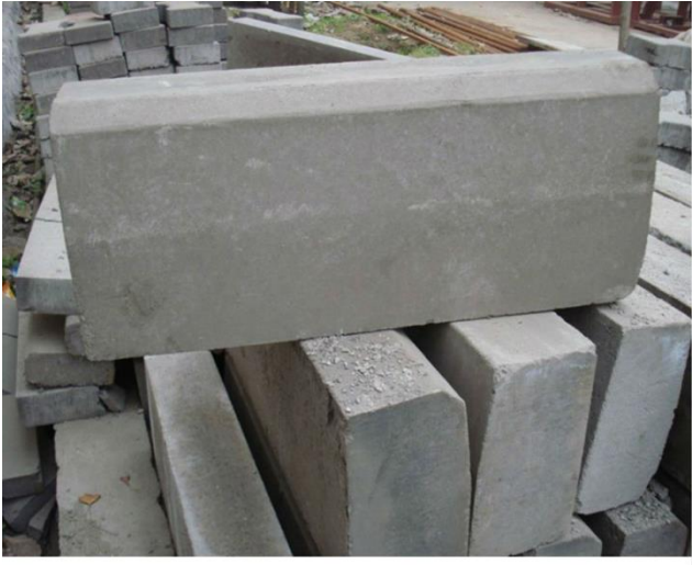
Figure 1.1: Barrier curb stone
