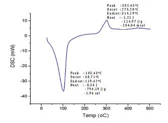
**Figure 4.** Thermal analysis (DSC) of bioplastic stone banana leaves powder/CMC/gum arabic on variation (55: 15: 30)%wt
