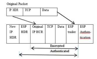
Figure 2. Authentication header in tunnel mode
