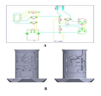
**Figure 2:** A) Battery Charging Circuit to be deformed and B) Both Sides of the Final Mechanical Representation.
