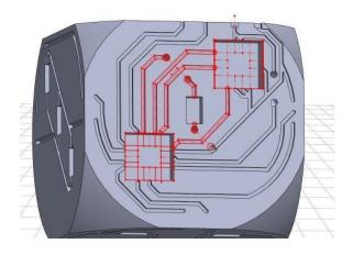
Figure 3: Electronic Circuit Mechanically Designed into Substrate.
