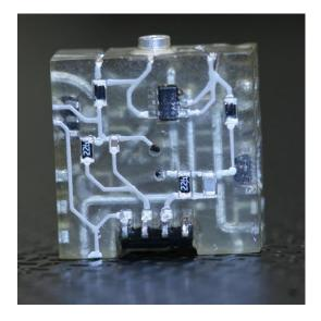
Figure 1: 3D Printed Signal Conditioning Circuit
